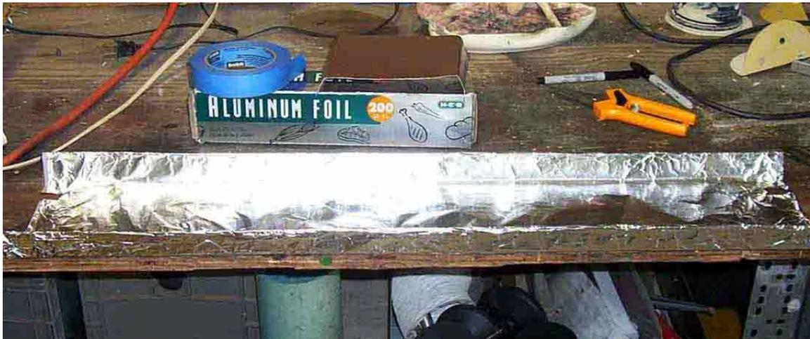
I made mine out of some 8" wide aluminum sheet metal that was (you guessed it!) laying around in my garage. I made the flat 5½" (width of my wood) and the flanges each 1¼" and wrapped it in good ol' HEB foil. Shiny side out, of course. Trim out 3 notches for your wires to pass through. Use duct tape liberally.
